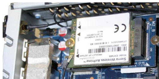
The installed riser card with additional LTE/4G card (top view) and SIM card (hidden). The pre-installed WLAN card and WLAN antenna must be removed before.
