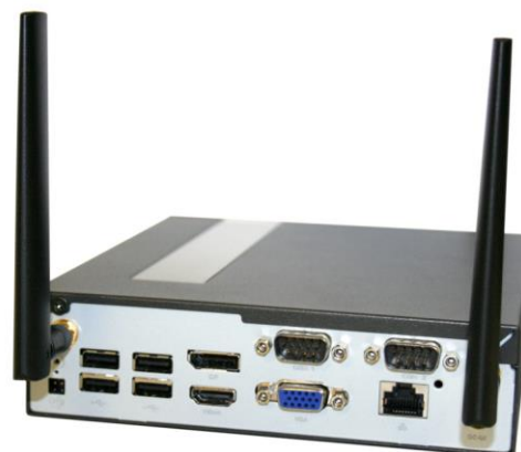
DL10J with installed cellular antennas.
