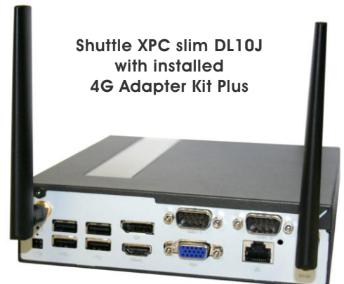
4G Antennas with Cables
