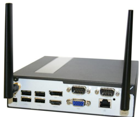
DL10J with installed cellular antennas.
